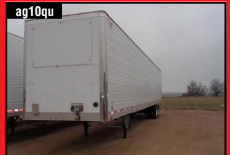
ag10qu 2016 Wabash 53' Reefer Air ride suspension, SS radius corners, SS Quilted doors, 24" Versitex Liner & Scuff, 5 lights top & bottom rails ..... Call
